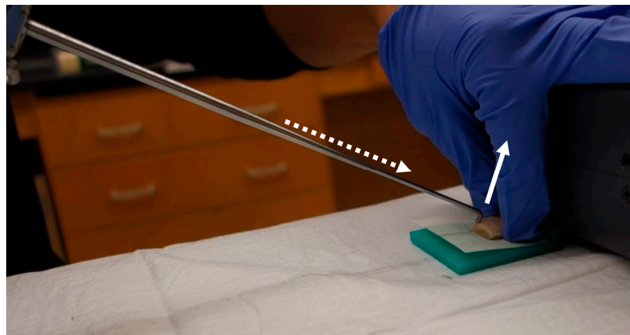
Figure 5. The sensor on the probe measured a reaction force (solid white arrow indicates its direction) on the cartilage surface while manually sliding the probe with 3 mm forward (white dotted arrow indicates its direction).
