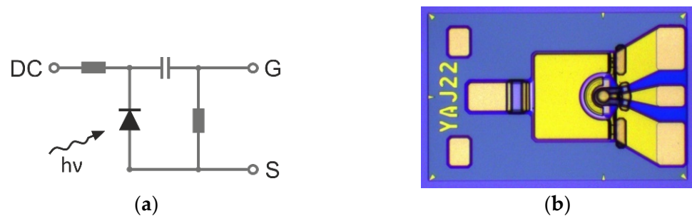
Figure 3. (a) Conceptual scheme of the photodetector chip. The resistor and the capacitor between the DC- and the ground-interface (G) implement the RC bias. The shunt resistor at the RF interface between the signal (S) and the ground (G) is the 50\ \Omega termination; (b) top view photograph of the processed photodetector chip.
