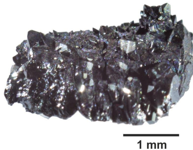
Figure 2. Crystalline hematite aggregate synthesized (conditions—450 °C, 1 kbar, NH 4 Cl solution).
