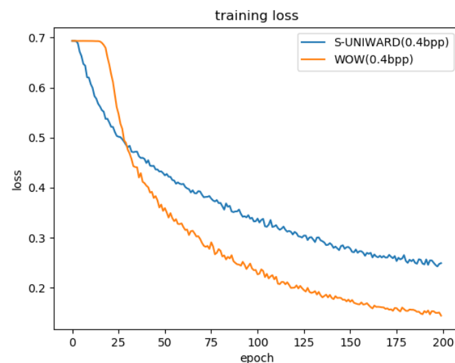
Figure 7. Comparing convergence performances of DFSE-Net against WOW and S-UNIWARD steganography algorithms at 0.4 bpp. Both models are trained and tested on the BOSS dataset.
