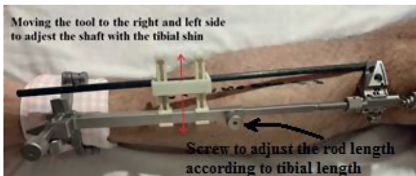
FIGURE 8: Fixing the tool properly.
