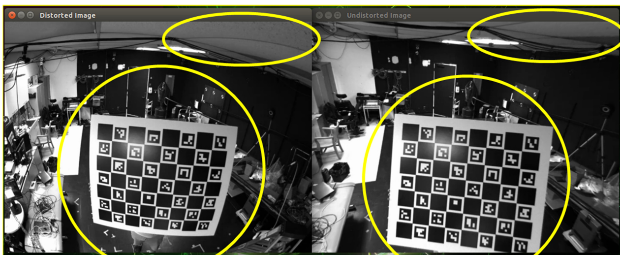
Figure A8. Barrel-distortion removal by camera-distortion model.
