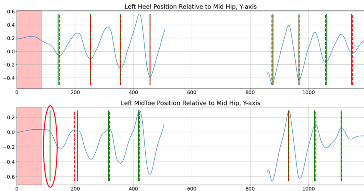
Figure 5. Foot-event detection. Solid green lines are ground-truth foot events, and dashed red lines are detected foot events. The solid green line circled in red shows an event that was missed but subsequently recovered using the IT recovery algorithm.
