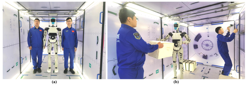
Figure 1. The robotic intravehicular assistant, Taikobot. (a) Taikobot is suspended in a space station mock-up. (b) A scenario where Taikobot helps astronauts transport cargoes with a dual arm system.
