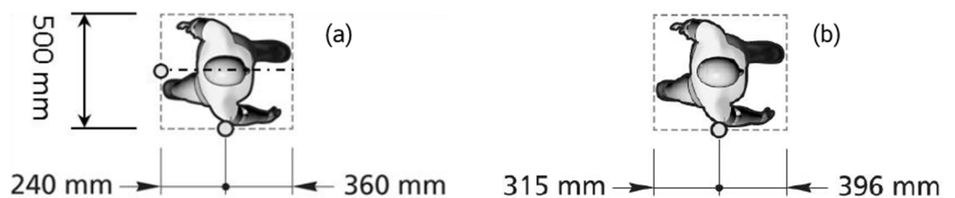
Figure 3. The bounding box for adult (a) and child pedestrian (b) dummy.
