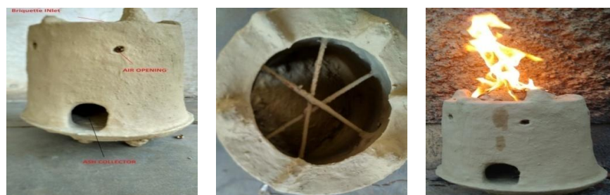
Fig. 6. Improved chulla/tandoor to suit with developed briquettes
