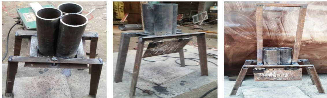
Fig. 4. Construction of low cost Briquetting machine
