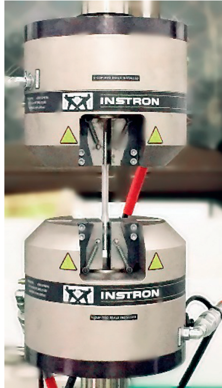
FIGURE 6: Fatigue testing setup.
