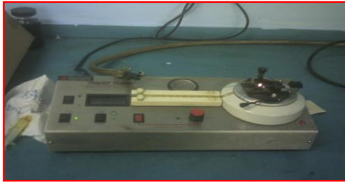
Fig. 6. Pensky-martens closed cup (PMCC) tester
