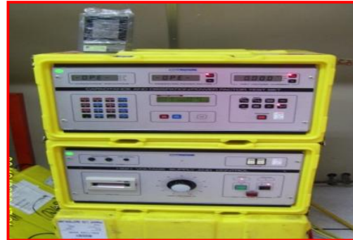
Fig. 3. Capacitance and dissipation / power factor test set and high voltage supply and control
