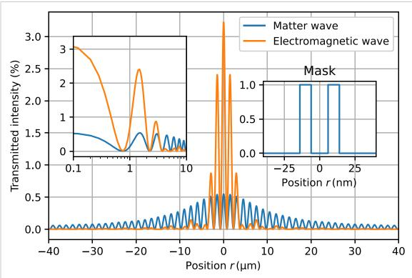
**Figure 7.** Comparison of the interference patterns obtained by passing a light wave (electromagnetic wave) (orange) and a metastable helium atom matter wave (blue) through the same SiN double-slit mask of 5 nm thickness with 8 nm openings separated by an 8 nm wall. The right inset shows the mask used for both cases. The left inset zooms into the first diffraction orders.
