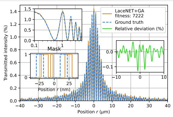
**Figure 8.** Pattern returned by the mask produced by LACENET after attempting to solve the double slit inversion problem. Note the near-perfect match with the ground truth despite the significant difference in the returned mask (lower left corner). The upper left inset shows the first diffraction orders, and the right inset (with the blue curve) depicts the deviation between the ground truth and the returned pattern in per cent.
