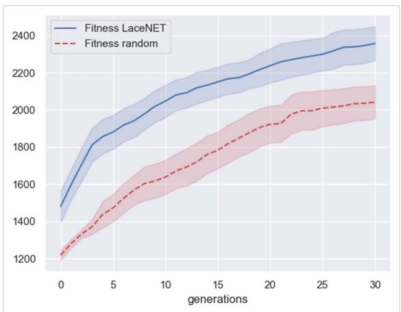
**Figure 5.** Average fitnesses F for an arbitrary mask after several generations of the genetic algorithm. The plot shows the solution's fitness when the initial population is given by LACENET (blue) compared with an initial population sampled randomly (red). Here is an example where LACENET helps to converge to a much more precise solution. Error bars (shaded area) are  $4\sigma$ , equivalent to 99.99% certainty.
