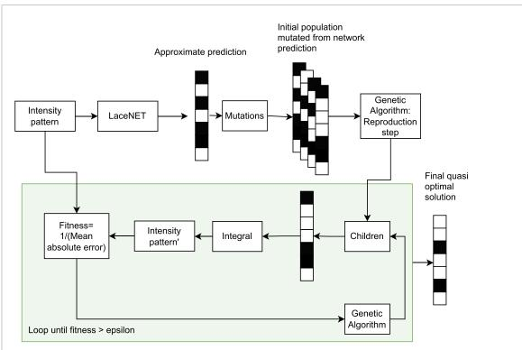
**Figure 1.** General mask generation framework used in this paper. First, the desired intensity pattern is fed to LACENET. LACENET then computes an approximated mask expected to produce this pattern. From this mask, an initial population is generated and fed to a genetic algorithm run until the accuracy condition is met.
