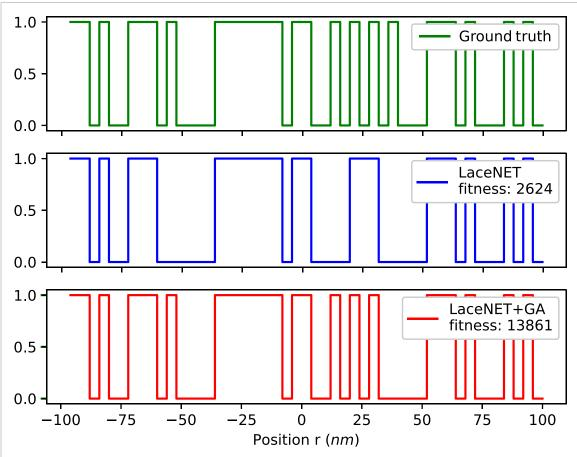
**Figure 6.** Example of a mask returned by LACENET (blue) and by LACENET enhanced by the genetic algorithm after 2000 generations compared (red) to the ground truth (green). Note how the genetic algorithm introduces certain openings in the mask that were missed by the neural network, thus increasing the general fitness of the solution. Note how LACENET (blue) also provides a reasonable first approximation to the mask design.
