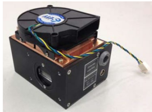
Figure 4. A photograph of the photon-counting PMT CH277.
