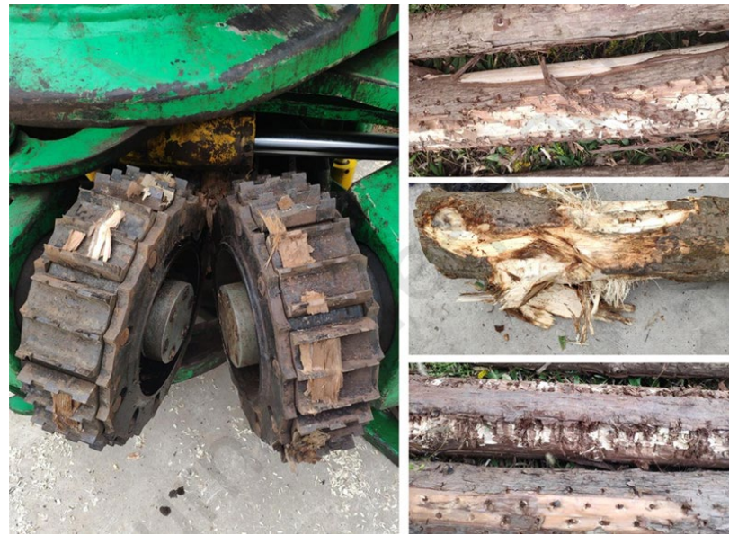
Figure 1. The damage to logs and the feeding roller of LAKO 43 forest harvester [7].
