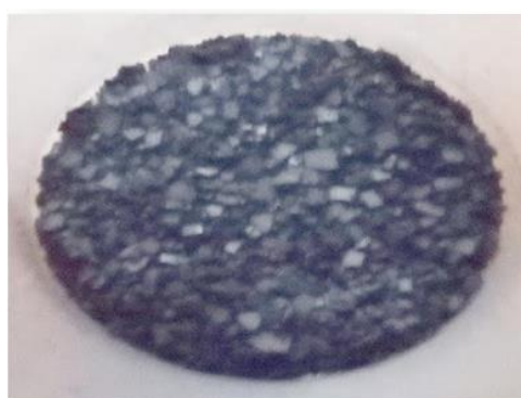
Fig. 7. Synthesized Plant-Ag-Graphene nanocomposites
