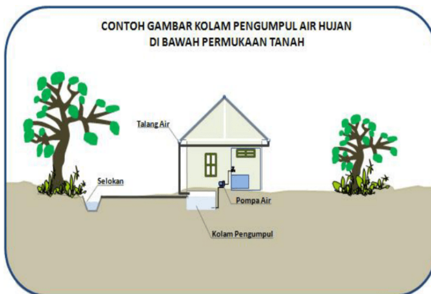
Fig. 4. Rainwater Collection Pond 1 (Example of a Picture of a Rainwater Collection Pond Below Ground Level)
