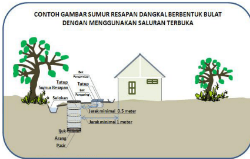
Fig. 3. Infiltration Well 2 (Example of A Picture of A Shallow, Round Infiltration Well Using an Open Channel)
