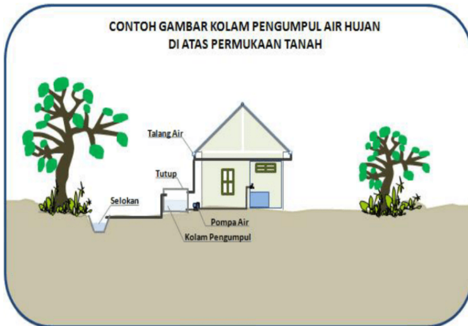
Fig. 5. Rainwater Collection Pond 2 (Example of a Picture of a Rainwater Collection Pond Above Ground Level)
