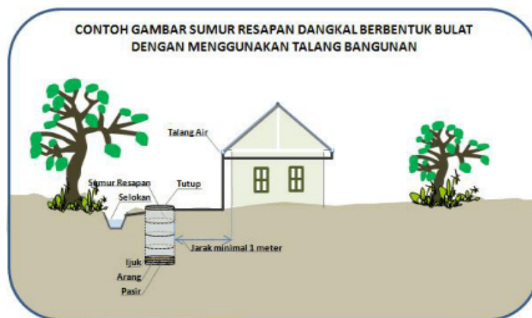
Fig. 2. Infiltration Well 1 (Example of A Picture of A Shallow, Round Infiltration Well Using A Building Gutter)
