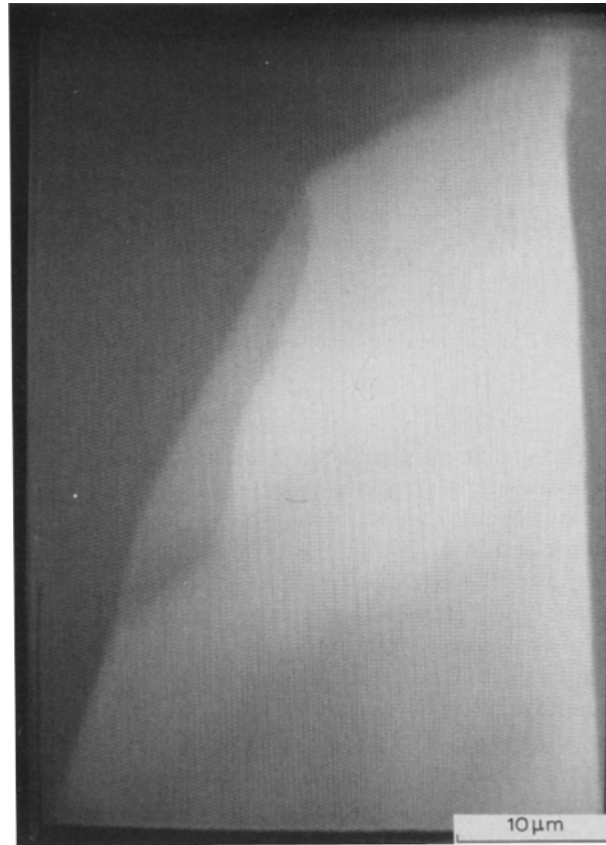
Figure 3. A bulge formed at a grain boundary of \beta -Ti6Al1-2V-6Zr alloy during rapid heating (photoemission electron microscope PEEM).
