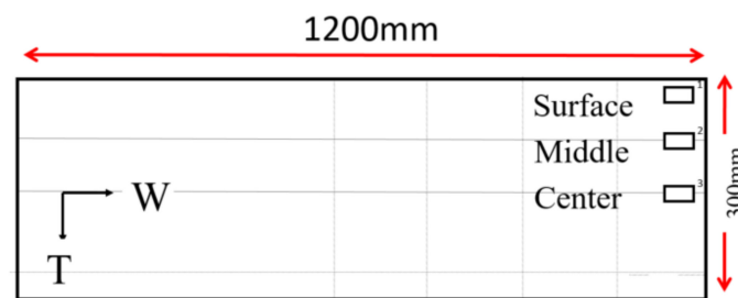
Figure 1. Sample positions in the ingot, W: width direction T: thickness direction.
