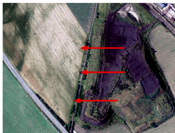
Figure 12. Dust coatings on the surface of arable soils surrounding the landfill.
