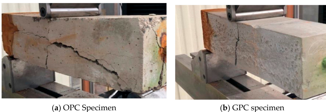
Figure 5. (a) OPC beam after 200 h of accelerated corrosion exposure, (b) GPC beam after 200 h accelerated corrosion exposure.
