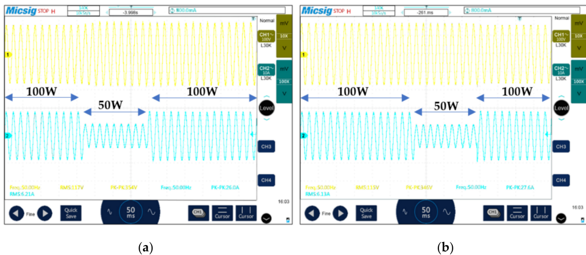
Figure 12. Load-Transient response for 100 W to 50 W step load change (Yellow—Output AC voltage, Blue—Output current): (a) Standalone 12 V–120 V inverter; (b) After applying the SCAWI-PV technique.
