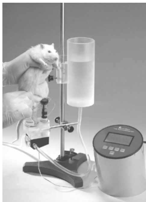
Fig. 2. Plethysmometer equipment used for rat paw edema model
