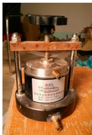
Figure 1. TST-55 permeameter. The TST-55 permeameter consisted of a cutting ring, two porous stones, a lantern ring, a top cover, a bottom cover, two rubber rings, and secured with bolts and nuts.
