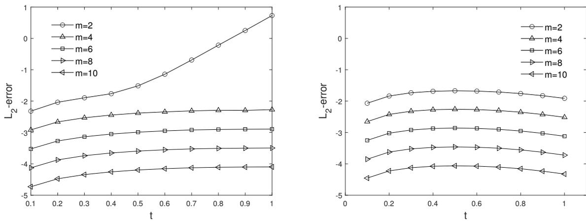
Figure 6.  $L_2$ —error using explicit method (left) and implicit error (right) taking  $r = 3$  and  $J = 2$  at time  $\delta t = 0.1/2^{m-1}$  for Example 2.
