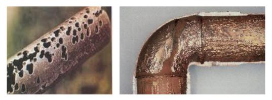
Plate 1. The effect of corrosion on metal pipes
