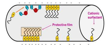
Plate 4. Adsorption of surfactants with polar heads and hydrophobic tails
