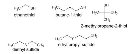
Fig. 4. Structures of additives used for odorization
