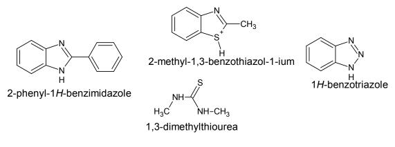
Fig. 5. The structure of corrosion inhibitors used in oil production
