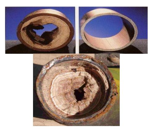
Plate 5. Scales formed in pipes
