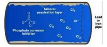
Plate 2. Phosphate corrosion inhibitors in pipes
