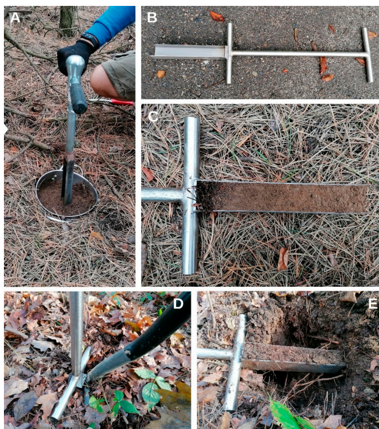
Figure 1. Litter and topsoil sampling: (A) mineral topsoil sampling using gouge auger in a site where first litter layer was sampled within a circle frame, (B) general view of a new sampler for joint litter + topsoil sampling, (C) jointly sampled litter + topsoil (0–25 cm), (D) cutting the soil sample with spade and digging the hole in a sampler's front, (E) the tilted sampler with the sampled topsoil.
