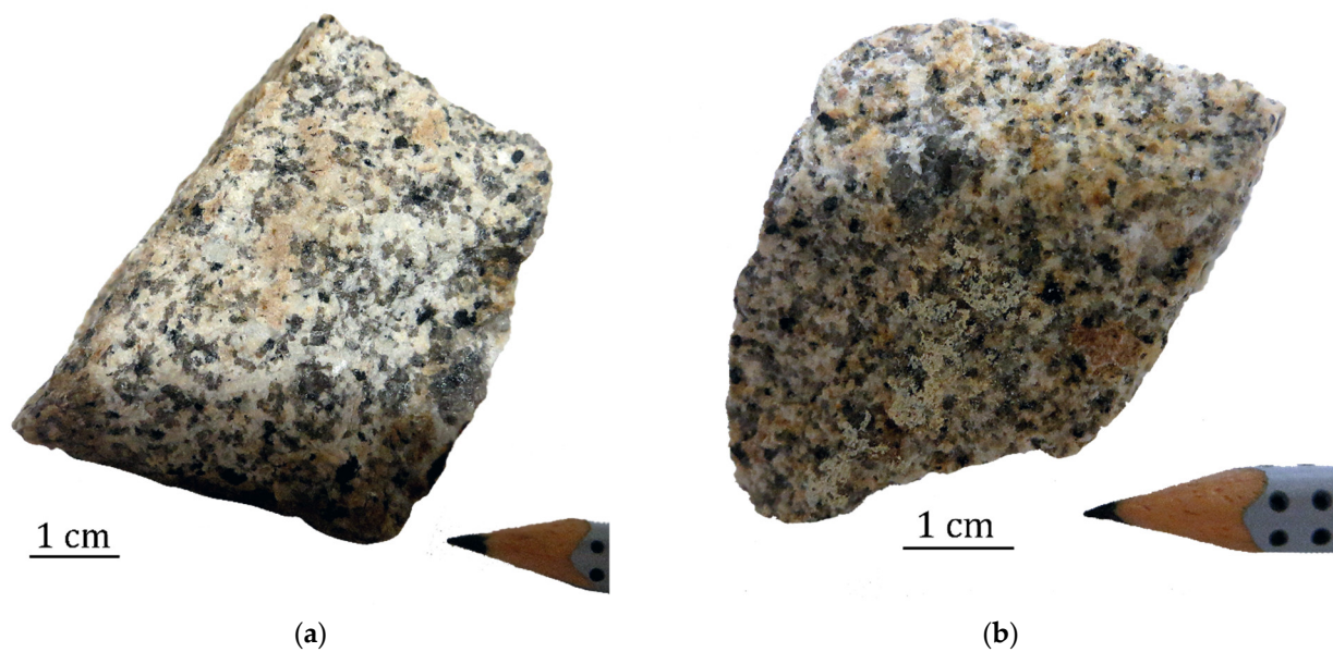
Figure 2. Chip samples of Li-F granites from Verkhneurmiysky massif: (a) medium-grained zinnwaldite granite; (b) medium-grained biotite granite.
