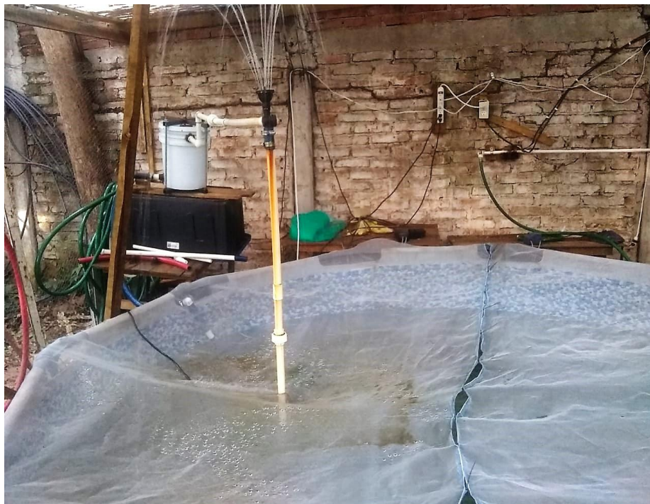
Fig. 3. Once the tilapias reached 24-26 g, they were transferred to a large pond (4678 liters) where remained until the end of experimental time. A submersible pump, an external filter and a device such as an inverted watering can, were used for filtering, recirculation and aeration the water
