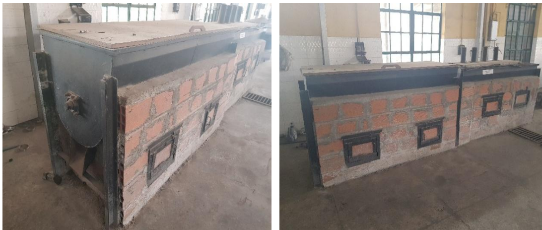
Plate 3a and b. Showing the discharge sprout and the side view of the power driven gari fryer
