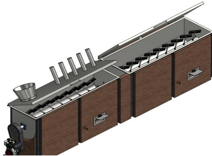
Figure 6. Isometric view of the fryer showing the paddles and inner part of the troughs
