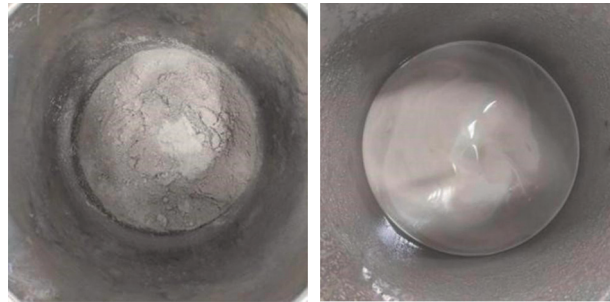
FIGURE 1: Sealing material before and after mixing.
