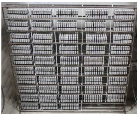
FIGURE 1: Some prepared PCC specimens.
