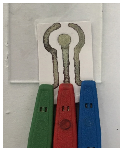
Figure 1. Indicates the connection of the designed three-electrode system by conductive Ag-ink (reference, working and counter electrode) to the electrochemical device
