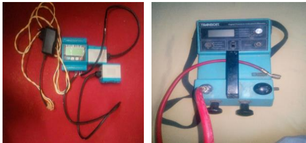
a) Ultrasonic flow meter b) Digital pressure indicator/calibrator
