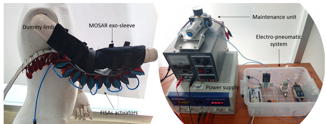
Figure 6. Experimental setup of FISAs above the MOSAR system with all the components.
