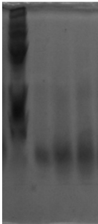
Fig. 2. SDS-PAGE electrophoretic pattern of laccase [homogenate (I); standart protein (bovine serum albumin, 66 kDa; egg ovalbumin, 45 kDa; pepsin, 34 kDa; trypsinogen, 29 kDa; carbonic anhydrase) (II); purified laccase enzyme from Russulaceae ( Lactarius volemus ) (III)]
