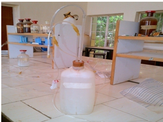
Plate 1. Set up for purification of carbon dioxide
