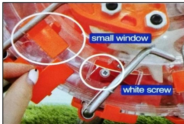
Fig. 2. Adjust the plant spacing
