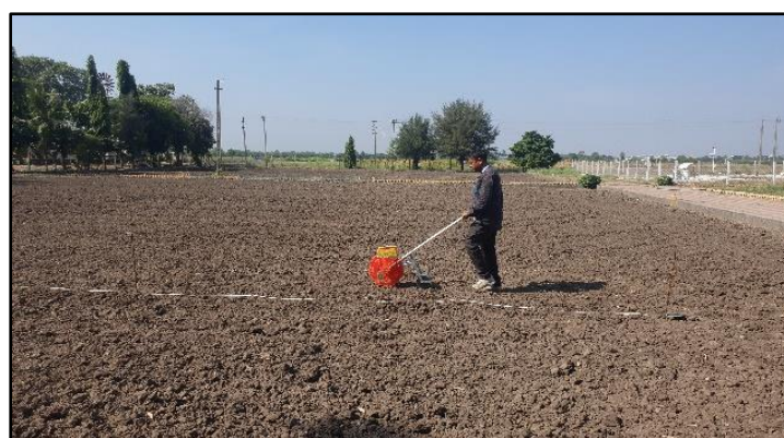
Fig. 5. Field testing of manual seeder
