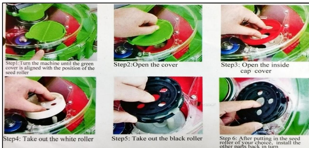
Fig. 3. Change the suitable seed roller
