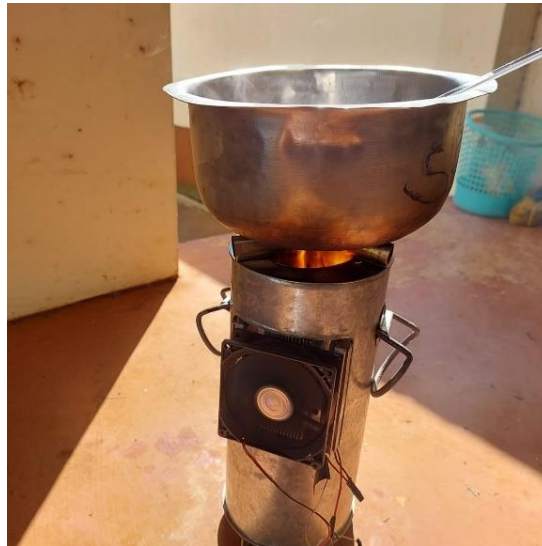
Fig. 8. TEG testing on the ICS
