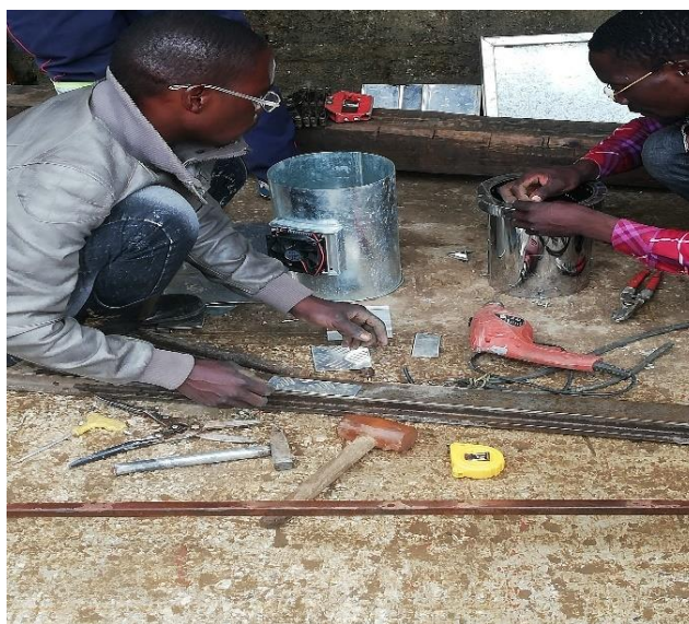
Fig. 7. Fabrication of outer casing and combustion chamber
