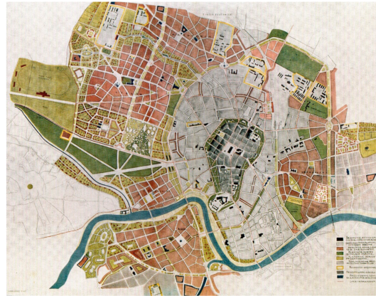
Figure 2. The Greater Cracow Regulation Plan—the winning competition entry by: Józef Czajkowski, Władysław Ekielski, Tadeusz Stryjeński, Ludwik Wojtyczko and Kazimierz Wyczyński, 1910, The creation of the urban form, extended beyond former fortifications of the inner city (everything that is marked differently than dark and light grey). The proposed layout, although never completed in that form, has been in many points repeated by the following urban plans of the city. source: reproduction in the collection of the Chair of Urbanism and City Structure Architecture of the CUT FA, photo by M. Nowak.
