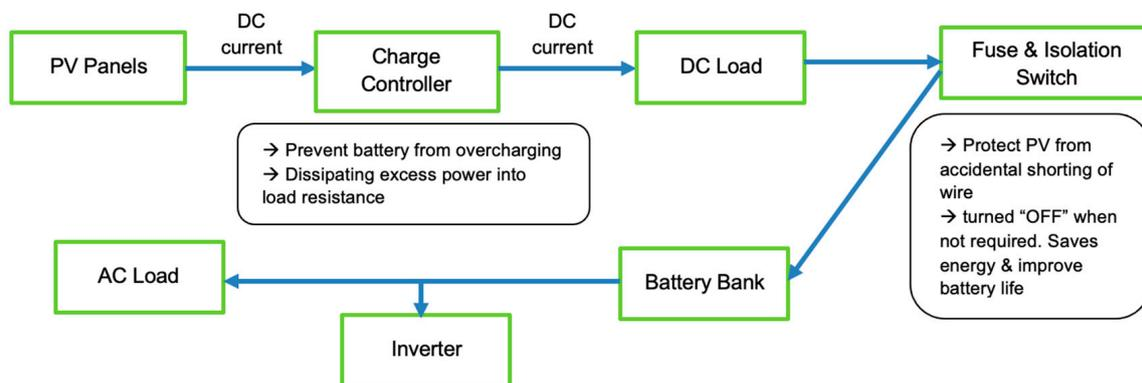
Figure 2. Solar standalone system balance-of-system (BOS).
