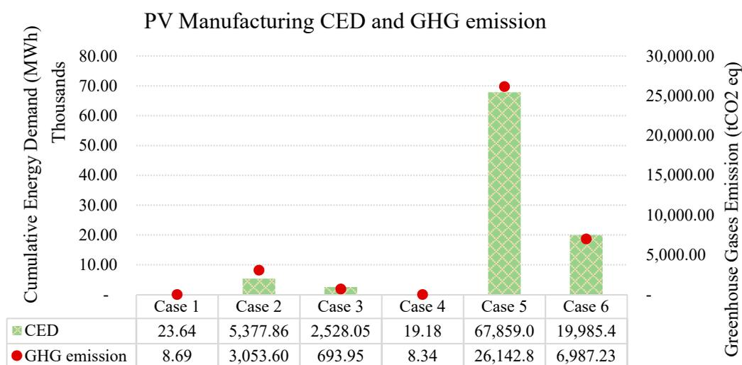
**Figure 10.** CED of different types of solar panel manufacturing and greenhouse gas (GHG) emission by case study.
