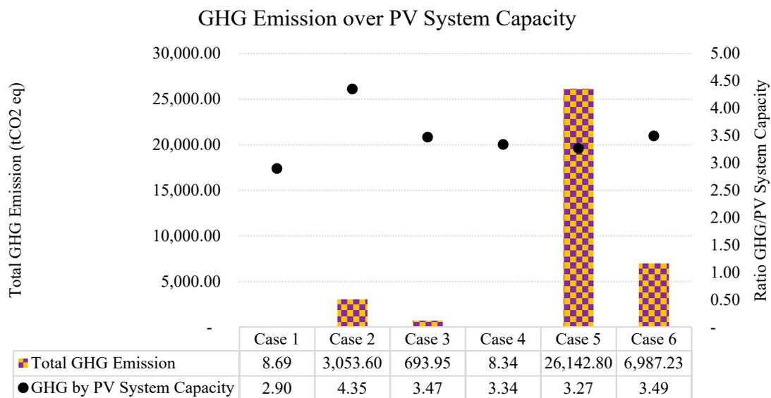
Figure 12. GHG emission normalized by PV system capacity.
