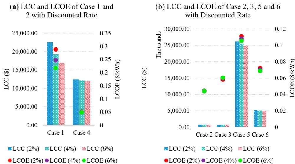
**Figure 14.** (a) Life cycle cost (LCC) and levelised cost of energy (LCOE) of case 1 and 4. (b) LCC and LCOE of case 2, 3, 5, and 6 based on different discount rates of 2%, 4%, and 6%.
