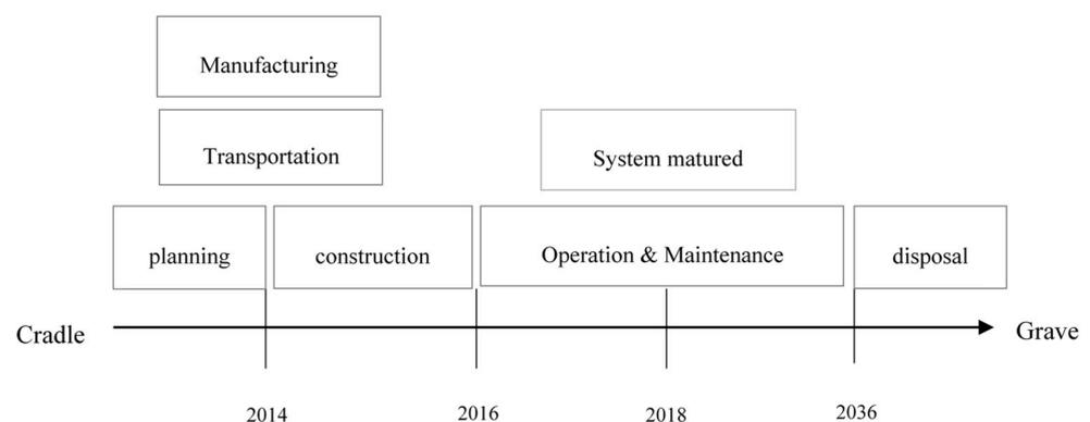
**Figure 1.** Photovoltaic (PV) systems life cycle timeline.
