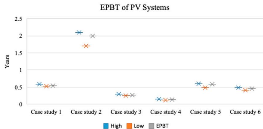
**Figure 11.** Energy payback time (EPBT) of PV systems varies based on maintenance energy investment.
