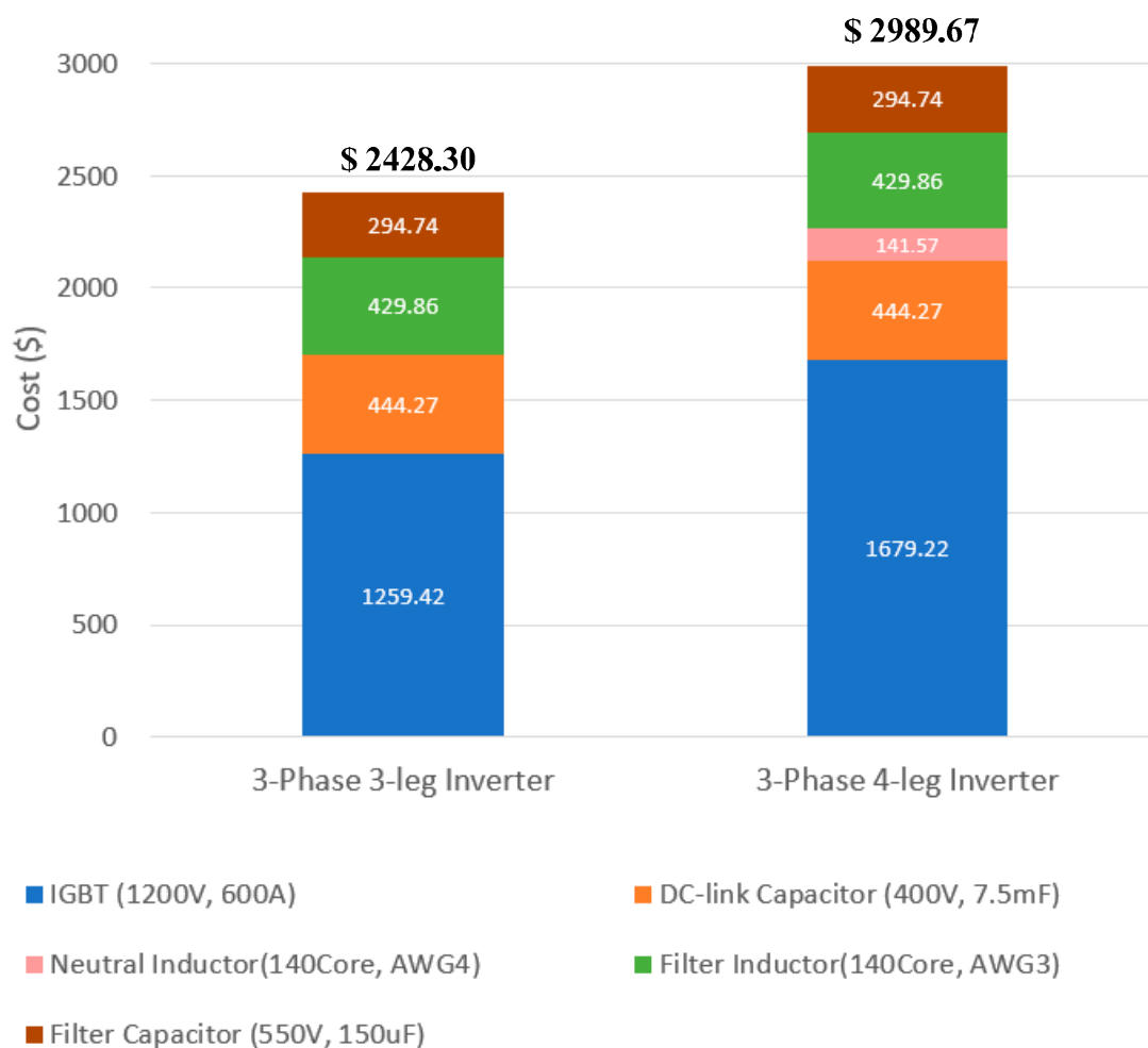
Figure 21. Cost comparison of 3-leg and 4-leg inverters using the cost model of the part.
