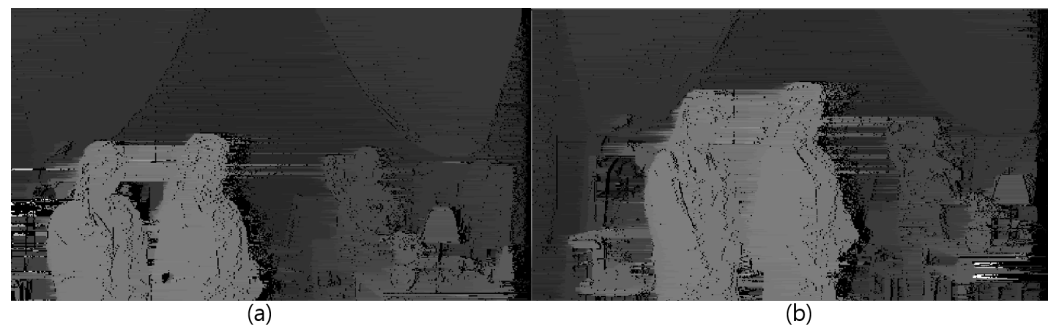
Figure 7. Two images with different scaling factors can be appropriately depth mapped from each perspective if the scaling factor is accurately estimated. (a,b) are the depth maps of the images of Figure 6a,b, respectively.
