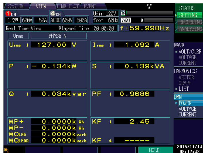
Figure 17. PF obtained in experimental tests of the power quality meter.
