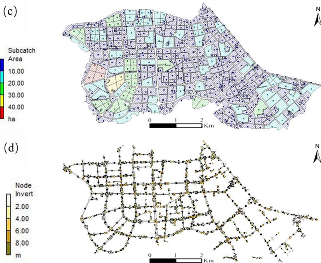
Figure 2. Key static variables and frames for Storm Water Management Model (SWMM). (a) DEM; (b) land use type; (c) sub-catchment of study area; (d) drainage system generalization of study area.
